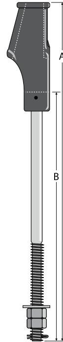
Each wedge socket consists of the socket, rod, wedge, 2 nuts, 1 washer, 1 cotter pin and 2 retaining clips.
