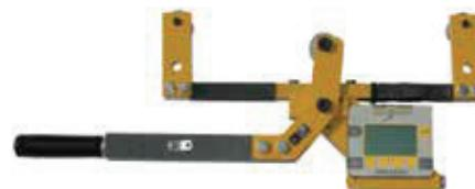
The Quick-Balance tension meter can be attached to a rope, used to measure tension and removed in just seconds. The digital load cell assures accuracy of up to +/- 3%. The meter is shipped from the factory with 1/2 in. • 12.7 mm, 9/16 in. • 14 mm and 5/8 in. • 16 mm diameter calibrations (other diameters are available by special order). The included sheave set accommodates wire diameters of 1/4 in. to 3/4 in.
