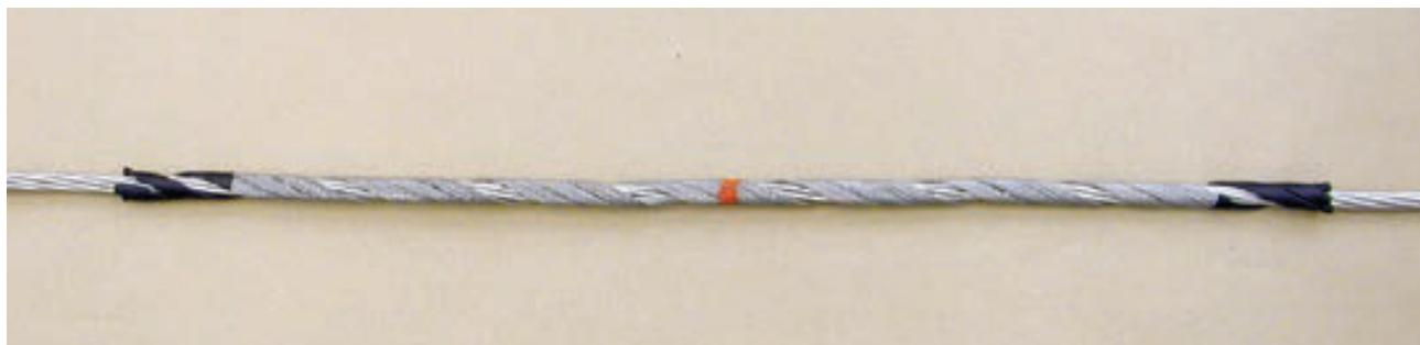
Note: Reeving Splices are not designed or intended for full strength applications. The purpose of their application is for replacing ropes, not for a permanent splice installation. Use ONLY once, then discard. Use ONLY for right lay ropes.
