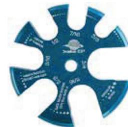
If the rope fits in the groove, or if a rope with rouge fits the stepped groove, retire the rope. Measurements based on ASME 17.6. Machined aluminum.
